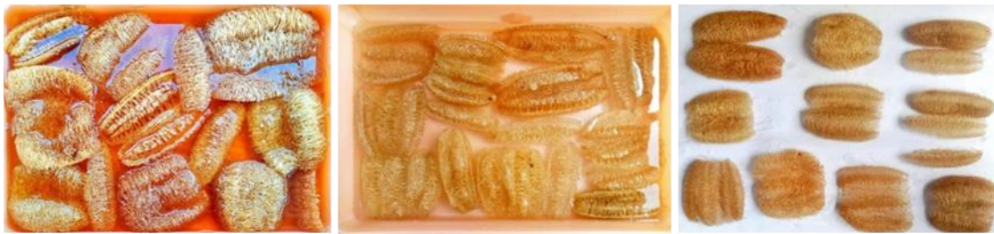
Fig. 1. Sodium acetate treatment of Luffa fibre
